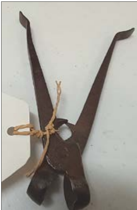
Early 19th century device for making lead shots for muskets. Photo Linda Rooney.
